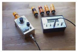
The sensitivity control affects the oscillator gain so there's maximum output near the middle of the tuning range but linearity is not particularly an issue. I still find a satisfying "dip" at the resonant frequency of whatever circuit It's coupled to. With any dip meter, you have to be careful not to over-couple the meter to the circuit you're testing. Too much load pulls the oscillator off frequency. The looser the coupling the more accurate the reading.
