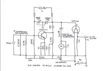
as it had sufficient frequency response. There's nothing critical about the choice of components. The asymmetrical tuning capacitor was lifted from a dead FM receiver. I haven't the foggiest idea what the capacitance range is but if you choose to duplicate this circuit, be sure the smaller tuning capacitor is connected to the base of the transistor. It won't work the other way round.
