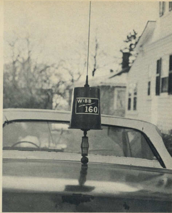
Whip antenna mounted on W1BB's auto. The loading coil is covered with a plastic trash can. Stew worked mobile on 160 meters for over 25 years, using both AM phone and CW.
