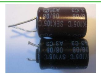
The capacitor on the bottom is pushing out the bottom plug.
